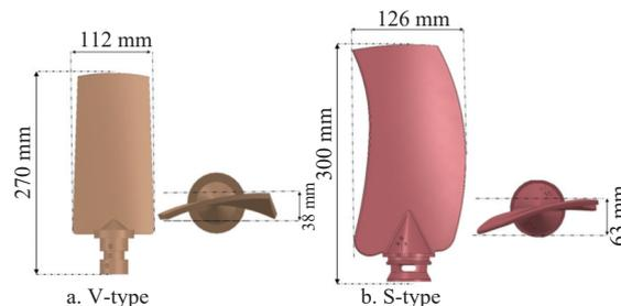
Figure 2 Side and top view of V-type and S-type fan blades
