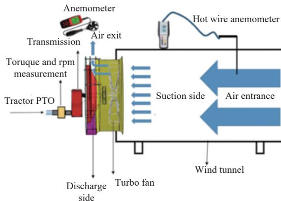
Figure 3 Schematic view of instrumentation and experimental positioning
