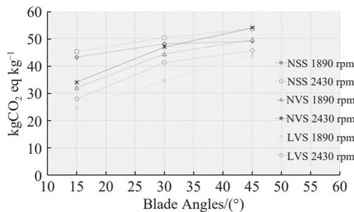
Figure 5 Carbon emissions (kgCO<sub>2</sub>eq/kg) at different blade angles and fan speeds
