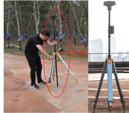
Figure 3 D-RTK 2 high-precision GNSS mobile station
