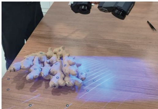
Figure 7 3D scanning modeling of ginger
