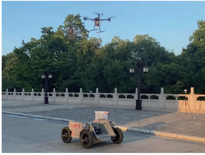
Figure 8 Formation control test of UAV-UGV
