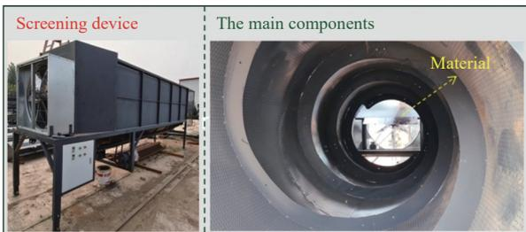
Figure 15 Material screening device
