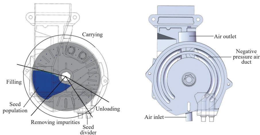
Figure 2 Working Flowchart of pneumatic double-disc precision seed metering device for Chinese flowering cabbage
