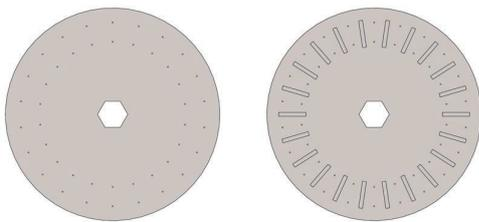
Figure 4 Seed discs of different specification
