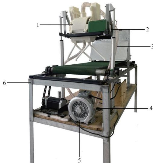
1.Pneumatic double disc precision seed metering device for Chinese flowering cabbage 2.Motor drive control device 3. PVC transparent steel wire pneumatic tube 4. pressure gauge 5. HG220 high-pressure vortex blower. 6. seeder performance test rig
