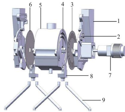
1. Seed box 2. Scrapers 3. Seed discs-1 4. Seeding shafts 5. Air chambers 6. Seed discs-2 7. Servo motor 8. Seed distributors 9. Seed guiding pipes
