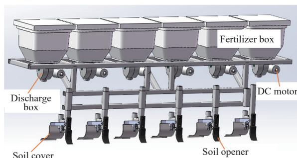
Figure 1 Six-row granular fertilizer applicator prototype
