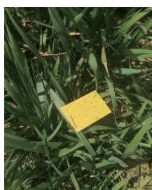
Figure 3 Water-sensitive paper placed on a leaf of wheat plot
