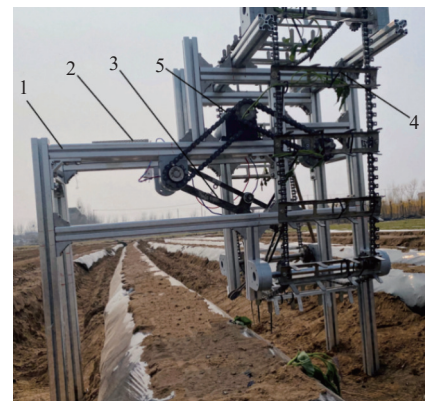
1. Rack 2. Switch power supply 3. Side insertion horizontal transplanting device 4. Seedling delivery device 5. 6D300-24 DC motor
