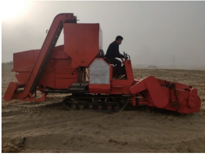
Figure 15 Verification of field operation of Cyperus esculentus combine harvester
