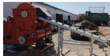
Figure 13 Operation validation of the wind sieve type cleaning device
