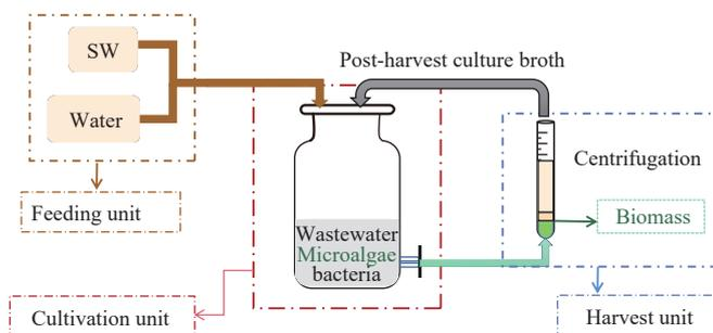
Figure 1 Schematic diagram of the recycling culture system
