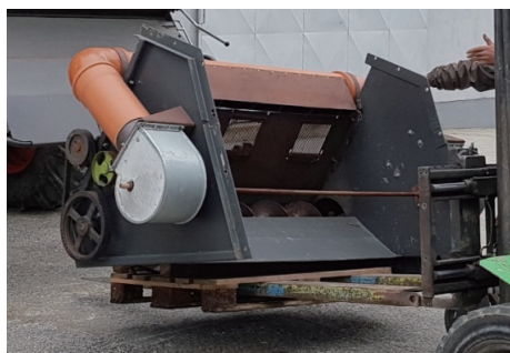
Figure 3 Assembly of additional cleaning fan, transport auger and grab container
