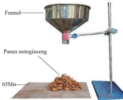
Figure 10 Stacking angle test
