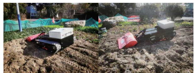
Figure 12 Experiment diagram of the working quality of the self-propelled electric tiller
