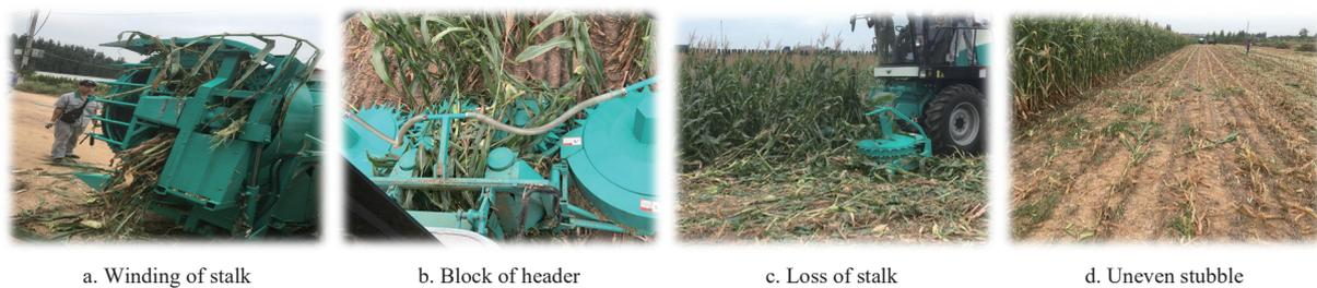
Figure 1 Production problems in the process of harvesting green forage maize
