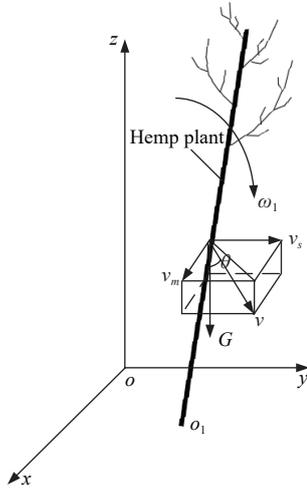
Figure 3 Analysis of landing process of hemp plants
