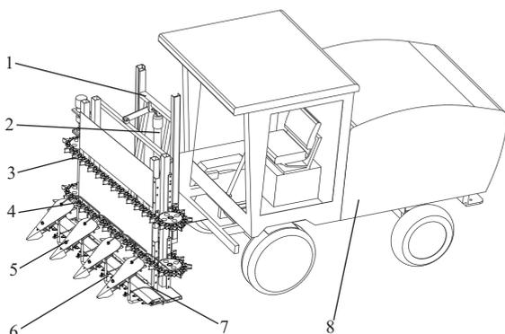
1.Header frame; 2.Header lifting cylinder; 3.Upper chain conveyor; 4.Lower chain conveyor; 5.Grain splitting and supporting device; 6.Double-knife reciprocating cutter 7.Pressure spring 8.Wheeled chassis
