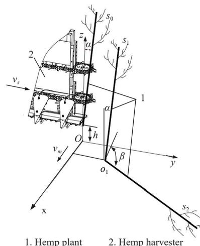
Figure 2 Schematic diagram of the hemp plant laying process
