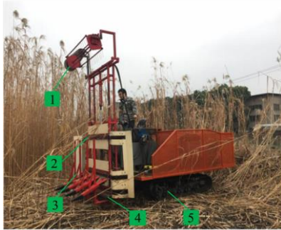
1. Upper stalk-guiding device 2. Three-layer chain conveyor 3. Lower stalk-splitting and stalk-holding device 4. Reciprocating double-acting cutter 5. Chassis system
