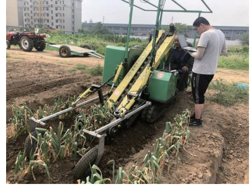
Figure 10 Field test of digging resistance
