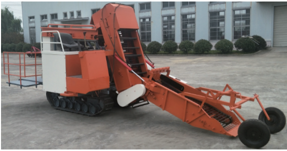
Figure 10 4UZL-1 sweet potato combine harvester
