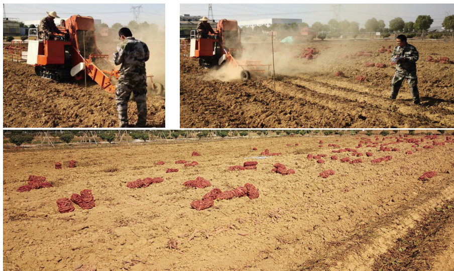
Figure 11 Field operation diagram of the 4UZL-1 sweet potato combine harvester
