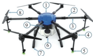
1. Flight Controller and Sensors 2. BLDC motor arm 3. Fluid hose pipe 4. BLDC Motor 5. Flat fan nozzle 6. Pesticide tank 7. Landing gear 8. Foldable propeller 9. LiPo Battery
