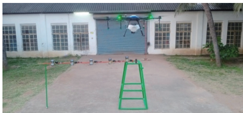
Figure 7 Experimental setup of multi rotor UAV downwash airflow pattern test at outdoor condition
