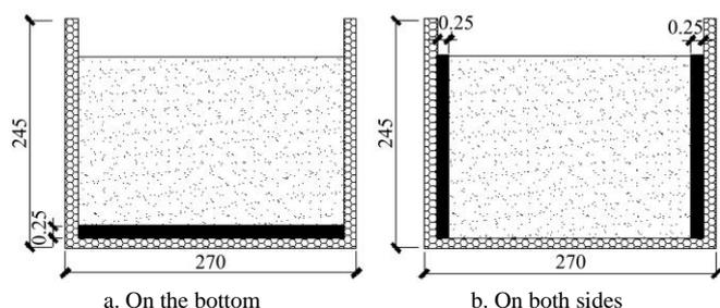
Figure 2 Different arrangement of carbon crystal electrothermal film
