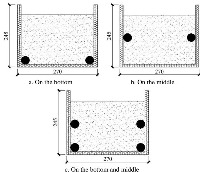
Figure 3 Different arrangement of low temperature hot water pipes
