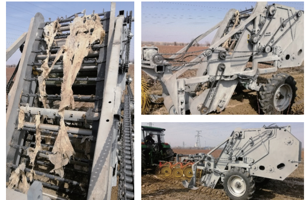
Figure 13 Field test of plastic film picking up device and its constituted recycle machine
