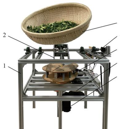
1. Frame 2. Shaking frame 3. Bamboo sieve 4. Hall angle sensor 5. Cam mechanism 6. Non-circular gear 7. Stepper motor
