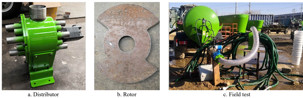
Figure 7 Photos of distributor, rotor, and field test
