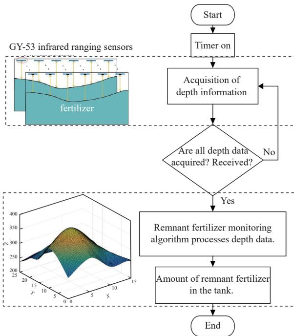
Figure 7 Depth information capture and parameter calculation
