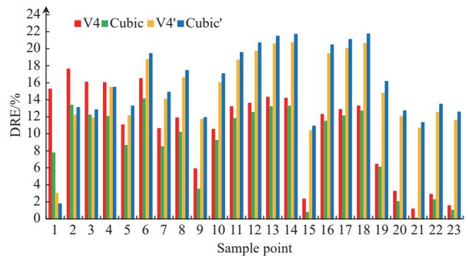
Figure 17 Relative error of discharged fertilizer monitoring in the field test
