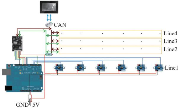
Figure 4 Connection diagram of the remnant fertilizer monitoring system
