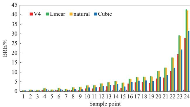
Figure 14 Relative error of remnant fertilizer monitoring in the bench test
