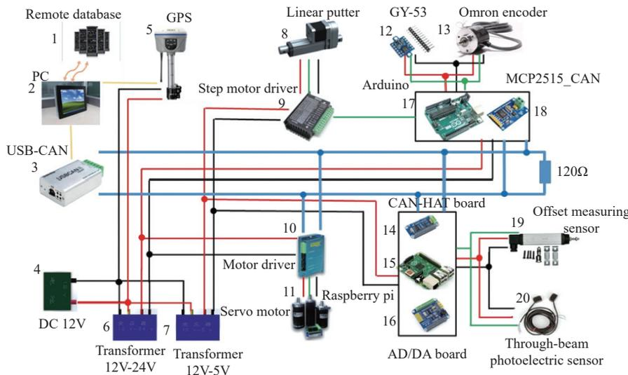
Figure 2 Connection diagram of the VRF system
