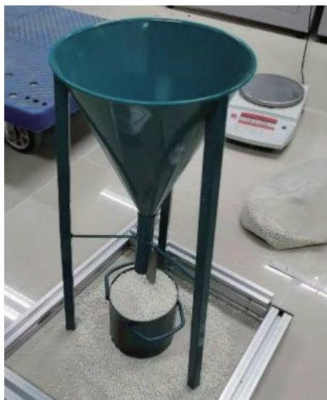
Figure 8 Calibration of the bulk density of the granular fertilizer
