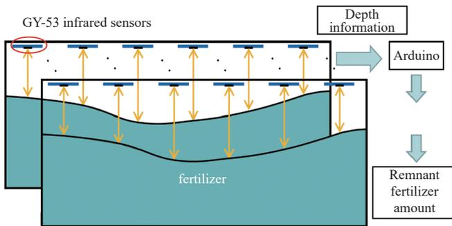
Figure 5 Working principle of the remnant fertilizer monitoring system
