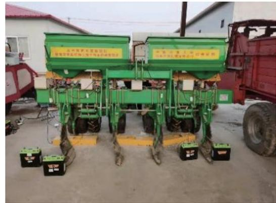
Figure 9 Bench test of the variable-rate fertilizer applicator and the remnant fertilizer monitoring system
