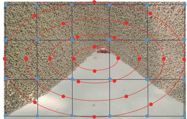
Figure 6 Depth information capture and parameter calculation (Red point and blue point are the GY-53 infrared sensors)
