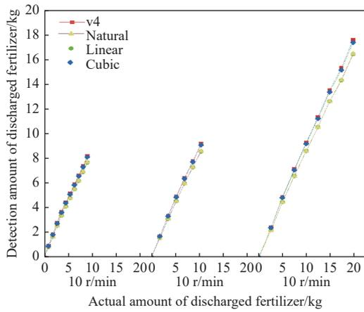
Figure 11 Actual and detection amounts of discharged fertilizer in the bench test
