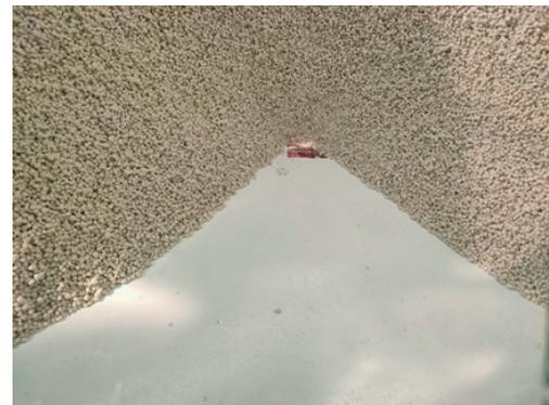
Figure 19 Shape of the fertilizer accumulation  $T=7$  min
