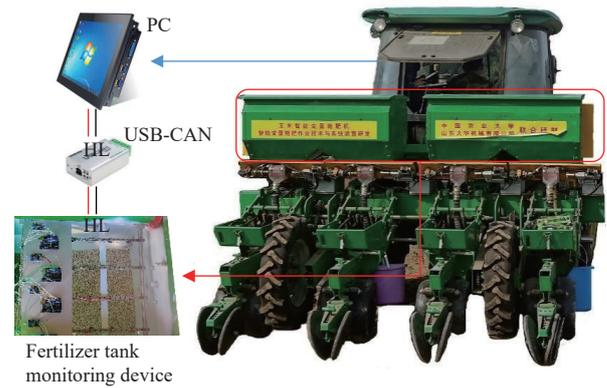
Figure 1 Framework of the remnant fertilizer monitoring system
