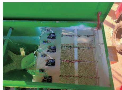
Figure 3 Remnant fertilizer monitoring device and its installation position
