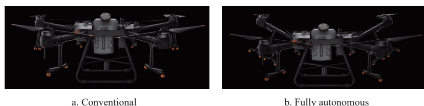
Figure 1 T30 model unmanned aerial vehicles in conventional and fully autonomous fruit tree spraying operation modes
