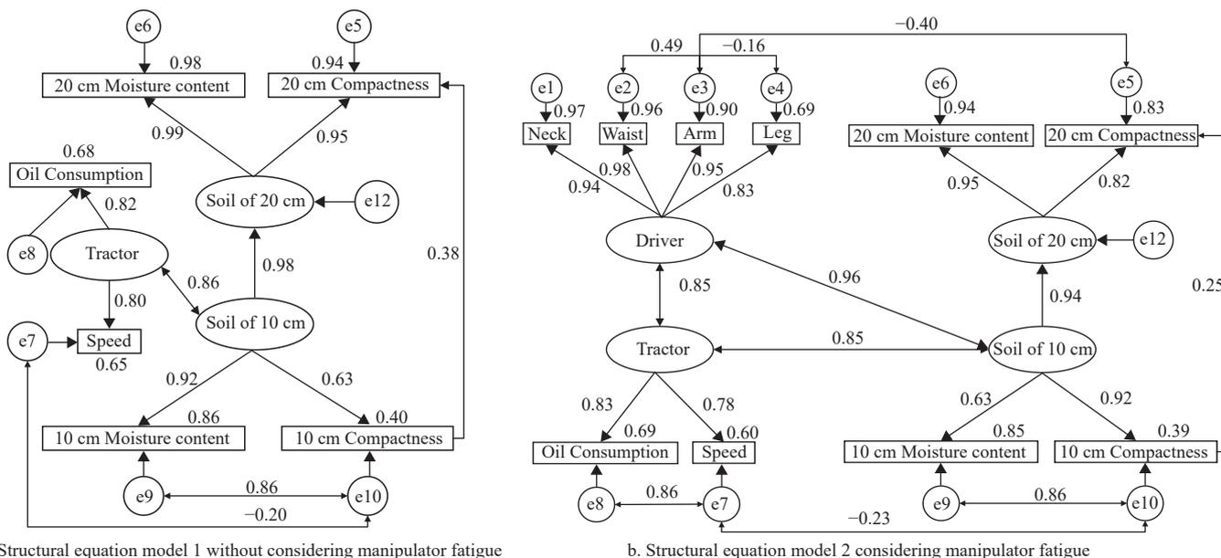
a. Structural equation model 1 without considering manipulator fatigue
