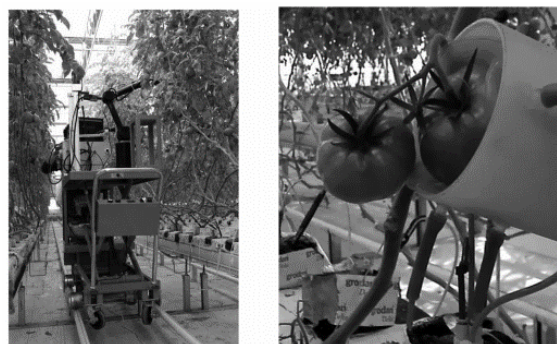
Figure 6 A tomato picking robot using adsorption
