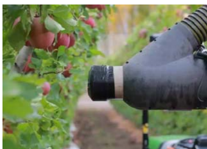
Figure 4 An apple harvesting robot using negative pressure adsorption
