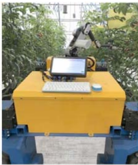
Figure 8 A tomato picking robot with double arms
