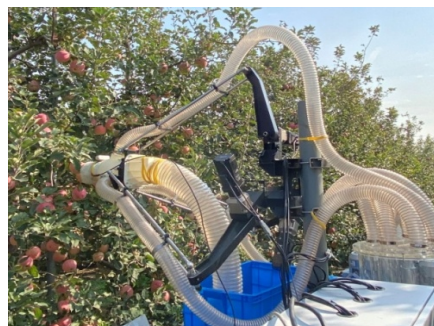
Figure 5 Another apple harvesting robot using negative pressure adsorption
