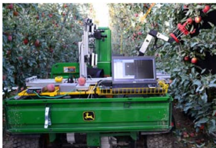
Figure 3 Fully automatic apple-picking robot using a shear force
