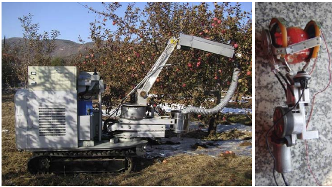
Figure 1 An apple-picking robot using a spoon-shaped end effector
