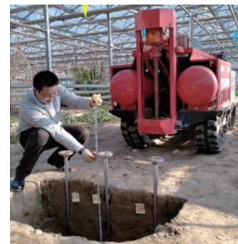
Figure 16 Observation and measurement of perforating profile of rods with different diameters
