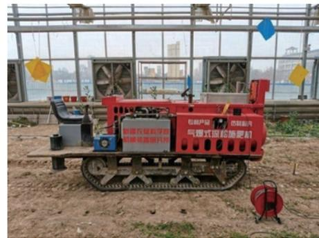
Figure 15 Gas explosion subsoiling and fertilizing machine and test site
