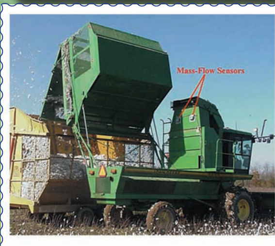
Figure 8 Two mass-flow sensors installed in a cotton stripper harvester
