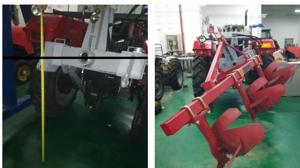
Figure 19 Tests of power lifting range and working slope range
