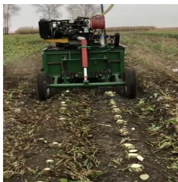
Figure 7 Sugar beet top cutting machine and cutting effect To obtain the highest qualified rate of top cutting and the
