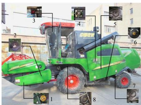
1. Cutter 2. Feeding auger 3. IPC 4. Threshing cylinder 5. Secondary Stirring 6. Rethresher 7. Vibrating Sieve 8. Conveyor chain harrow
