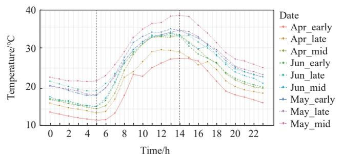
Figure 6 Variation trend of hourly temperature in Solar Greenhouse
