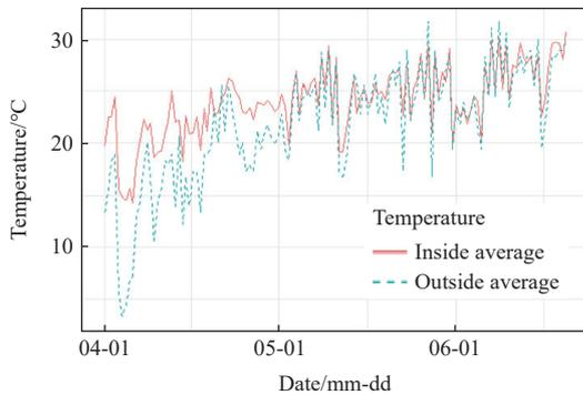
Figure 2 Comparison of average temperature trend of the year 2017-2018 inside and outside the greenhouse
