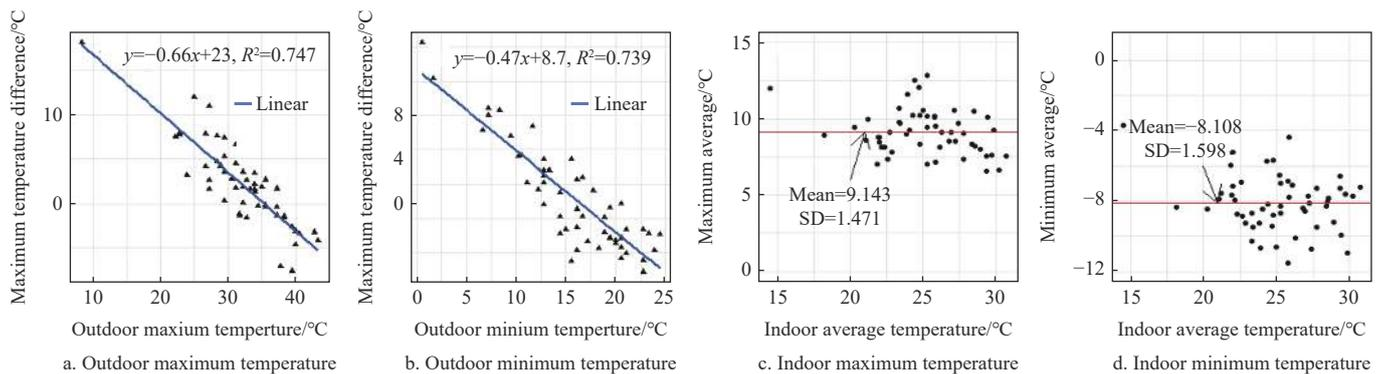
Figure 5 Correlation Analysis of indoor and outdoor maximum and minimum temperatures
