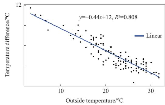
Figure 3 Daily average temperature difference versus outdoor temperature
