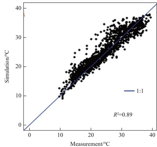
Figure 9 Simulated temperature plotted against measurement for 1801 h data from March to June over the years of 2017 and 2018
