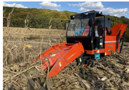
b. Juming 4YZLP-2C crawler style self-propelled corn ear harvester (JM-2C harvester)
