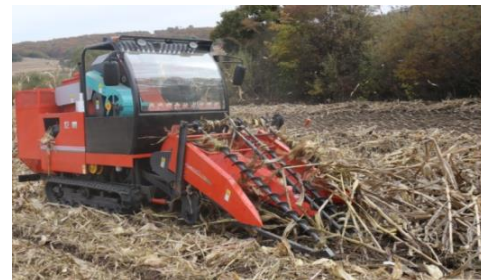
c. Juming 4YZLP-2C crawler harvester equipped with spiral auxiliary feeding device for lodged corn (JM-2CAF)
