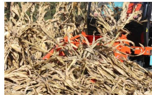
a. Head blockage of the JM-2C harvester
