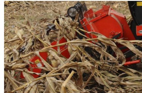
b. Stalks fracture on the JM-2CAF harvester
