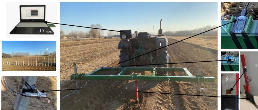
1. Tractor 2. Data acquisition card 3. Differential amplifier 4. Fertilizing shovel 5. Wheatstone-bridge strain gauge 6. Three-point suspension and frame 7. Compacted soil 8. Laser sensor 9. Reflection strips 10. Laptop
