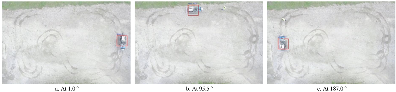
Figure 3 Images taken by a DJI MAVIC 2 drone used as ground truth with three different orientations of the robot
