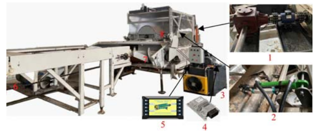
1. Reducer and dynamic torque sensor 2. Hydraulic cylinder and displacement sensor 3. Hydraulic station 4. Controller 5. Human-machine interface 6. Chain conveyor 7. Feeding device 8. Threshing device
