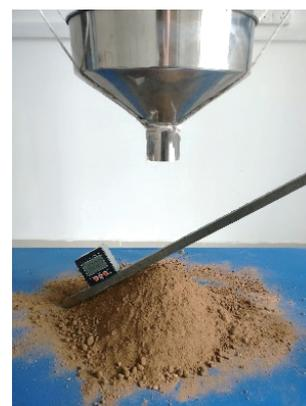
Figure 3 Repose angle test
