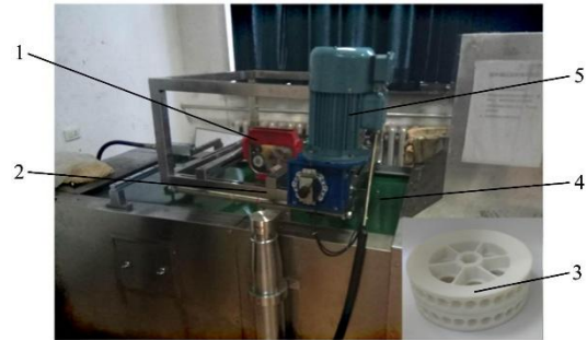
1. Soybean hole wheel seeding device 2. Mounting rack 3. Hole seed-metering wheels in contrast groups 4. Belt of seed bed 5. Motor
