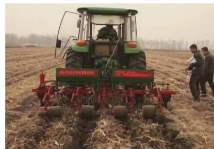
Figure 6 Experiment in field of subsoiling and variable rate fertilization machine
