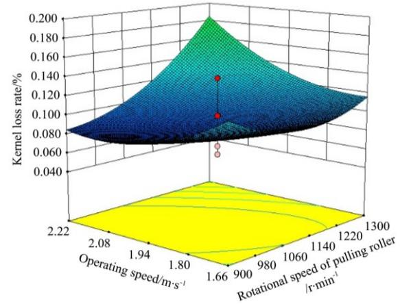
a. Interaction of rotational speed of pulling roller and operating speed
