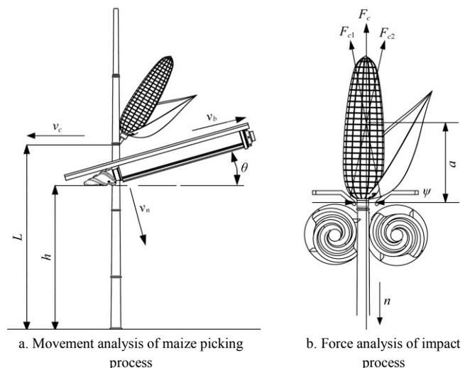
Figure 1 Mechanism analysis of maize picking process
