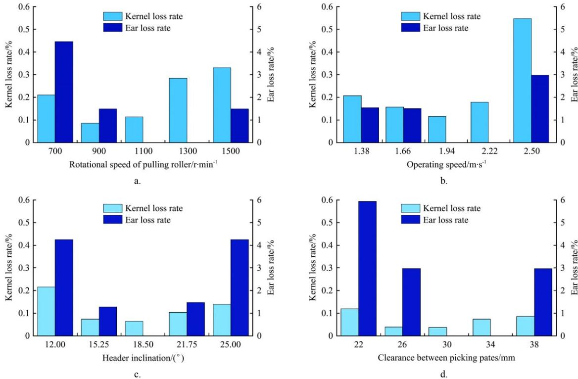
Figure 5 Effects of different operating parameters on maize picking performance
