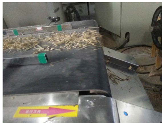
b. Kernel-MOG mixture falling onto the sensor
