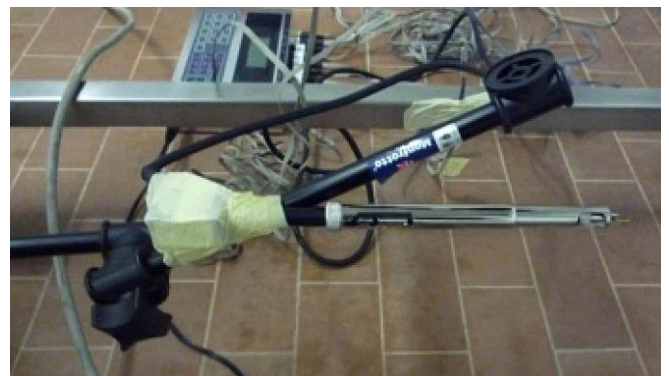
Figure 9 Anemometer (central, 23 cm from floor)
