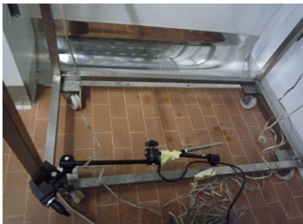
Figure 12 Anemometer (50 cm from lateral panel; 23 cm from floor)
