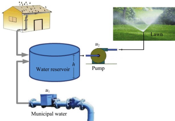
Figure 1 Schematic of rooftop water harvesting (RWH) for lawn irrigation [61]
