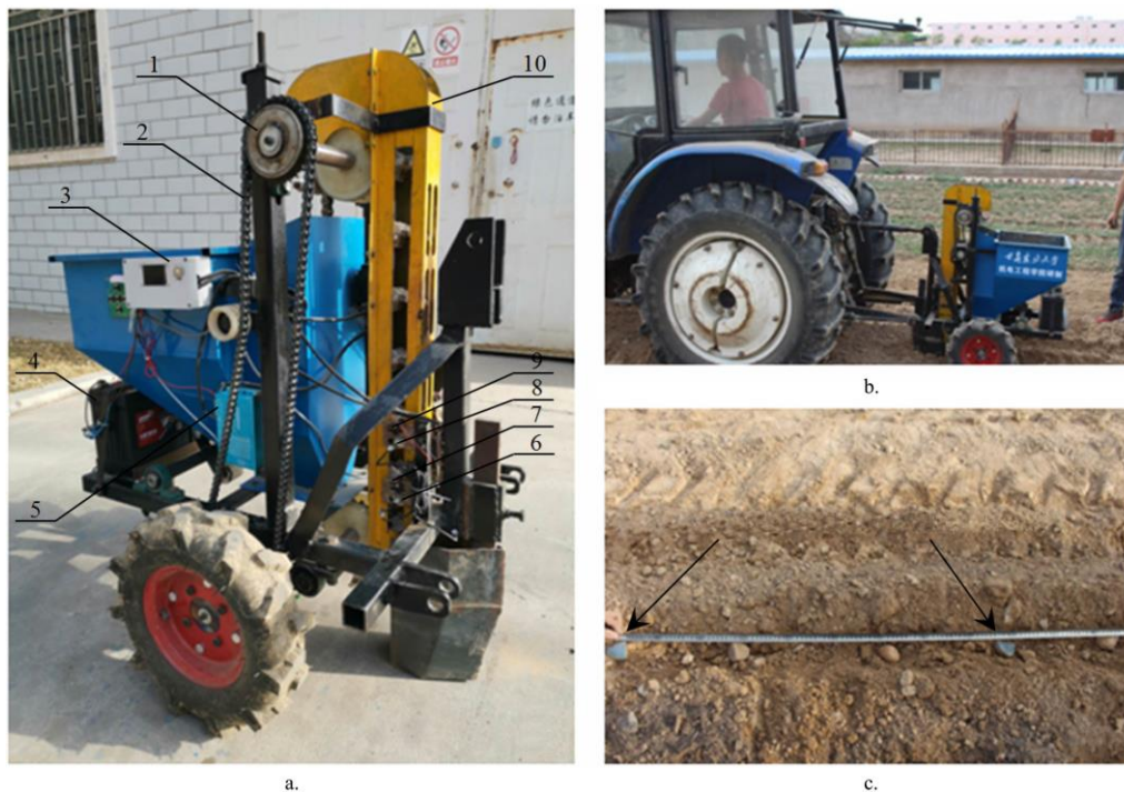
1. Main power transmission one-way clutch 2. Land wheel power transmission chain 3. System controller 4. Vehicle battery 5. Electric motor driver 6. Seed spoon position sensor I 7. Photoelectric sensor set for seed-metering detection I 8. Seed spoon position sensor II 9. Photoelectric sensor set for seed-metering detection II 10. Seed-metering groove.
