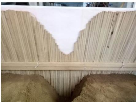
Figure 3 Soil disturbance measurement using a profile meter in an excavated furrow
