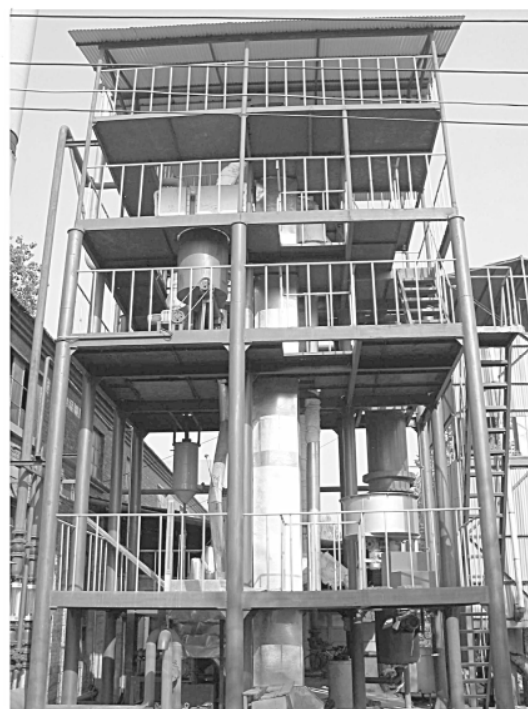
Figure 3 Pilot plant of ceramic ball heated down-flow tuber reactor for fast pyrolysis of corn stover to produce bio-oil funded by 863 Program
