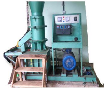
Figure 1 Die and roller machine used in co-compost pelletization
