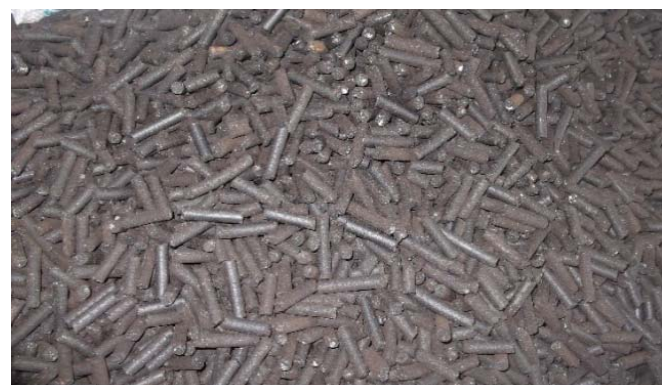
Figure 4 Compost Pellets made with co-compost (MSW+ FS) of PC1 particles and 25% moisture using die and roll pelletizer
