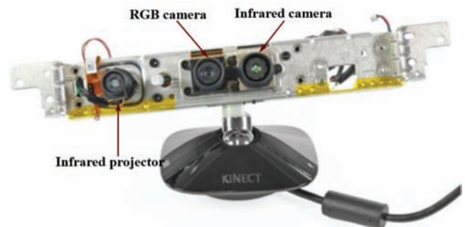
Figure 2 Inside structure of the Kinect sensor, the infrared (IR) projector, IR camera, and RGB camera.
